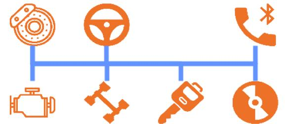
Figure 4: Network topology with single line bus
