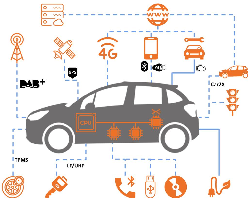
Figure 1: Overview of external interfaces on modern cars
