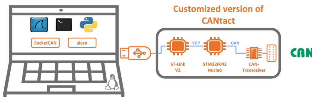
Figure 2: Functional diagram of the CANtact penetration testing framework
