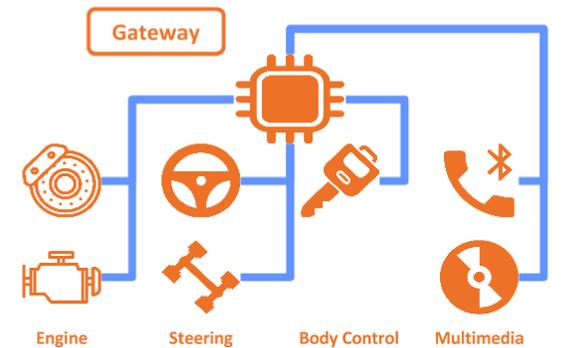
Figure 3: Network topology with central gateway
